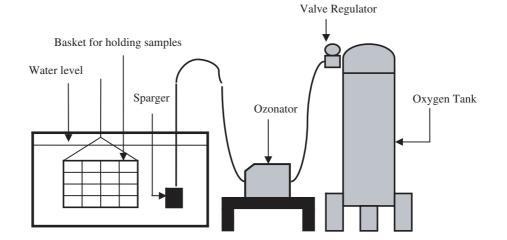
Figure 1 The schematic of ozonator for produce ozonated water.
